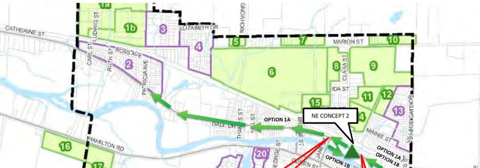
Deep Trunk Sewer Alternative requires that sewer be constructed at up to 4 metres deeper than if a PS is constructed to service area. Localized sections of the Deep Trunk Sewer can be nearly 10 metres deep
