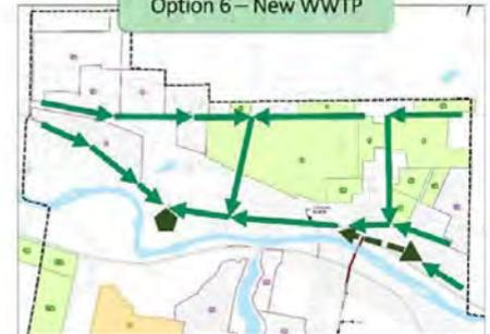
→ Gravity Sewer    - - - Forcemain    ▲ Pumping Station    ■ Treatment Plant
