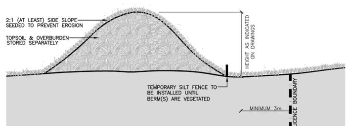
TYPICAL BERM SECTION N.T.S.
