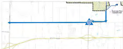
Servicing Concept 3 – Supply 401 Corridor Lands with BPS + Fire Pump
